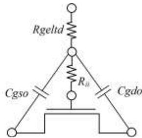
In this case, the gate electrode resistance given by (9.10) is in series with the intrinsic-input resistance  $R_{ii}$  as given by (9.6) through two internal gate nodes, so that the overlap capacitance current will not pass through the intrinsic-input resistance. *trnqsMod* = 0 (default) and *acnqsMod* = 0 (default) should be selected for this case.
