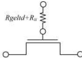
In this case, the gate resistance is the sum of the electrode gate resistance (9.10) and the intrinsic-input resistance  $R_{ii}$  as given by (9.6). An internal gate node will be generated.  $trnqsMod = 0$  (default) and  $acnqsMod = 0$  (default) should be selected for this case.
