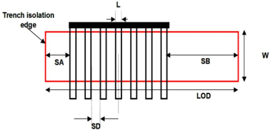
Figure 14.3 Layout of multiple finger MOSFET
