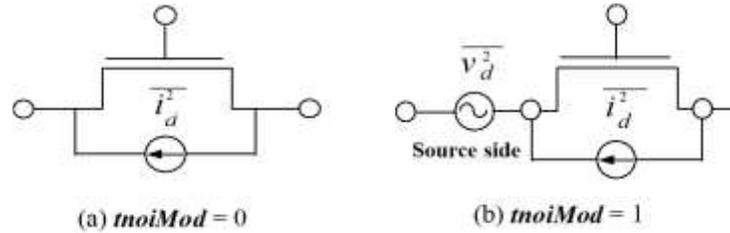
**Figure 10.1 Schematic for BSIM4 channel thermal noise modeling.**
