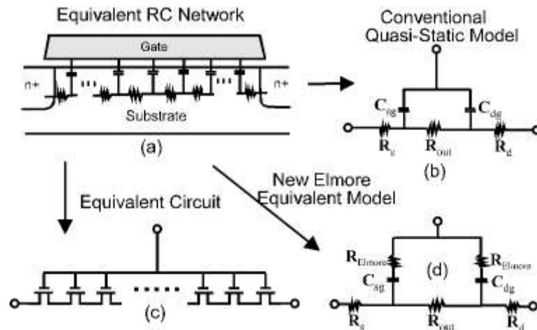
**Figure 9.1 Quasi-Static and Non-Quasi-Static models for SPICE analysis.**
