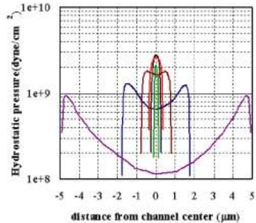
**Figure 14.2 Stress distribution within MOSFET channel using 2D simulation**
