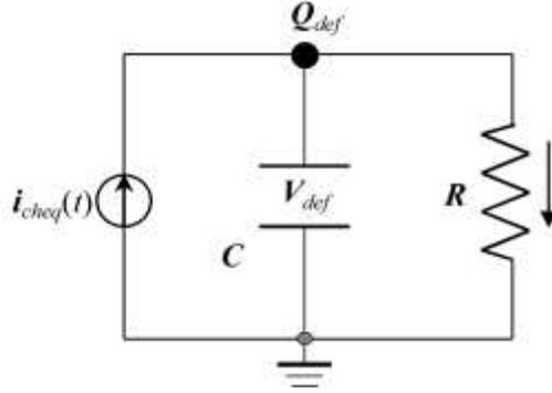
**Figure 9.2 Charge deficit NQS sub-circuit for transient analysis.**
