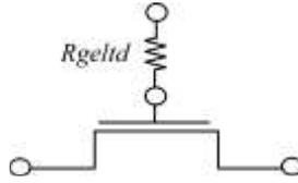
In this case, only the electrode gate resistance (bias-independent) is generated by adding an internal gate node.  $R_{geltd}$  is given by
