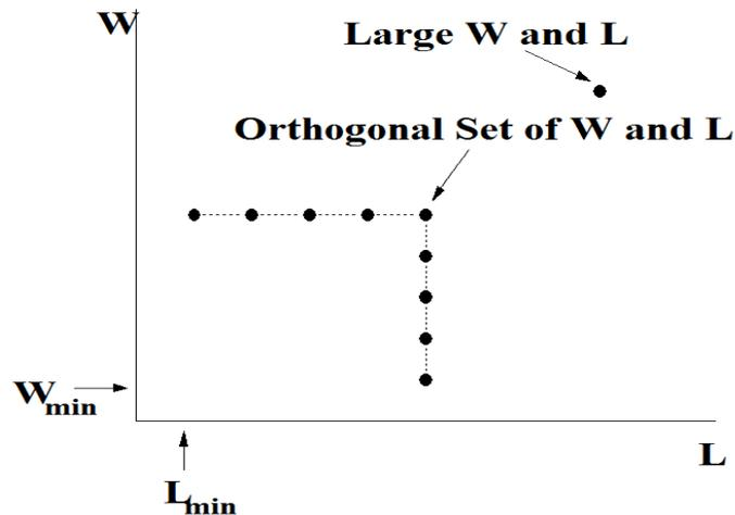
**Figure 16.1** Device geometries used for parameter extraction
