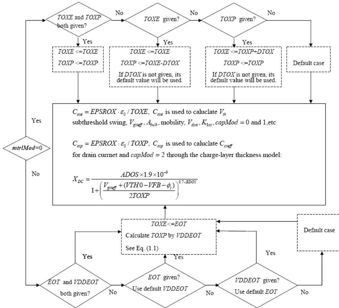
**Figure 1.1 Algorithm for BSIM4 gate dielectric model.**
