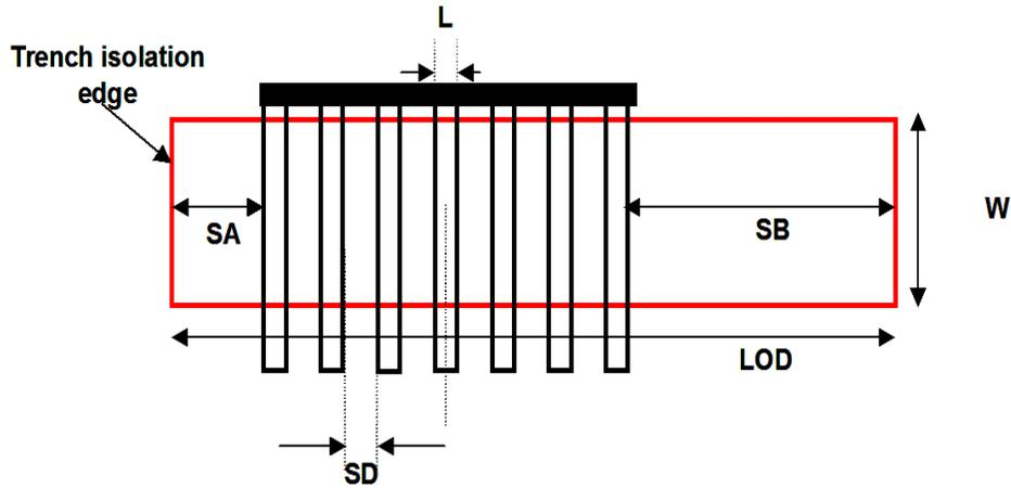
Figure 14.3 Layout of multiple finger MOSFET
