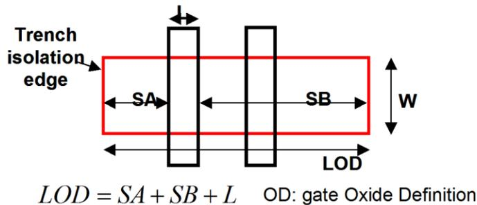
**Figure 14.1 shows the typical layout of a MOSFET**
