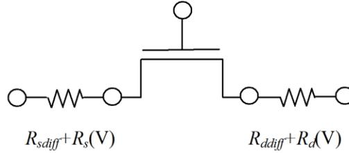
The diffusion source/drain resistance  $R_{sdiff}$  and  $R_{ddiff}$  models are given in the chapter of layout-dependence models.
